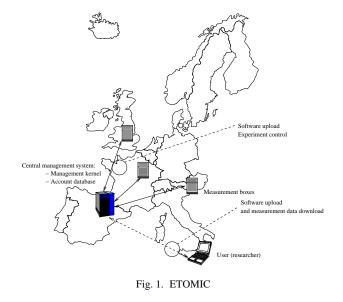
The system components are depicted in figure 1. A central management system is in charge of system control, comprising not only the scheduling and execution of measurements experiments, but also system monitoring (survivability) and configuration. The central management system is composed by a workstation and a traffic repository to which measurements can
