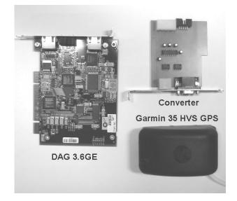
Fig. 2. DAG 3.6GE, GPS and converter
