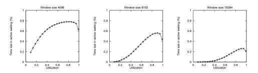
Figure 4. Percentage of transaction delay lost in active waiting for window sizes of 4 KB, 8 KB and 16 KB
