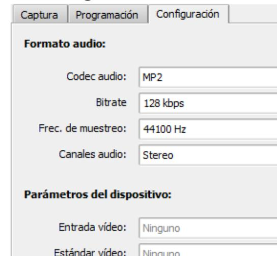
The screenshot shows a software interface with three tabs: 'Captura', 'Programación', and 'Configuración'. The 'Configuración' tab is active. Under the heading 'Formato audio:', there are four settings: 'Codec audio:' set to 'MP2', 'Bitrate' set to '128 kbps', 'Frec. de muestreo:' set to '44100 Hz', and 'Canales audio:' set to 'Stereo'. Below this, under the heading 'Parámetros del dispositivo:', there are two settings: 'Entrada vídeo:' set to 'Ninguno' and 'Estándar vídeo:' set to 'Ninguno'.
