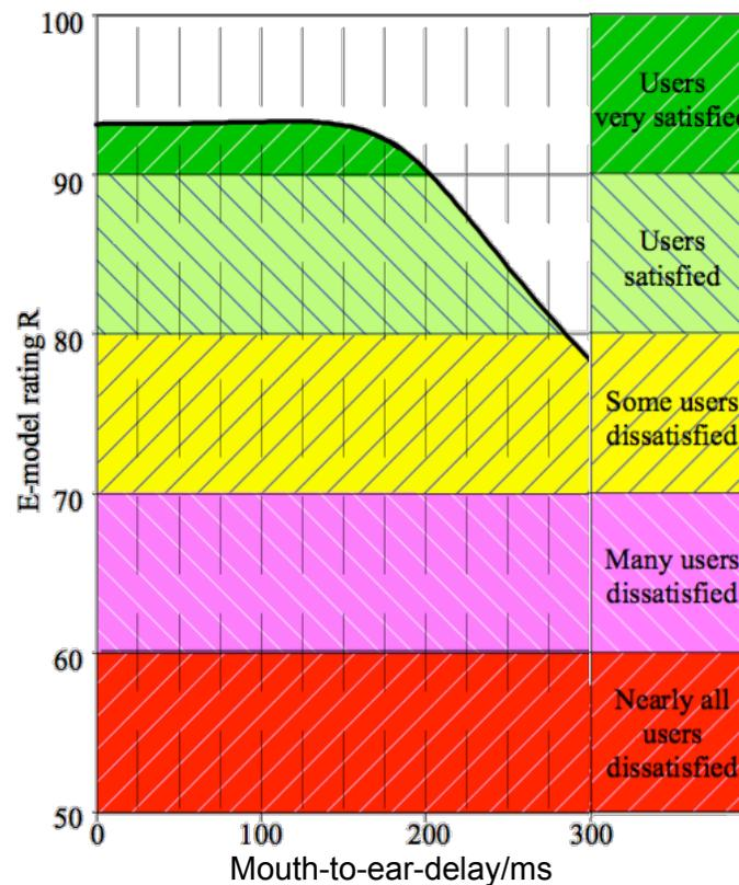
Figure 1/G.114 – Determination of the effects of absolute delay by the E-model
