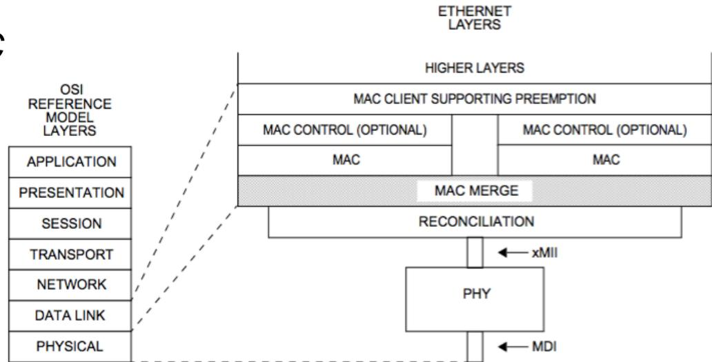
NOTE—In this figure, the xMII is used as a generic term for the Media Independent Interfaces for implementations of 100 Mb/s and above. For example: for 100 Mb/s implementations this interface is called MII; for 1 Gb/s implementations it is called GMII; for 10 Gb/s implementations it is called XGMII; etc.
