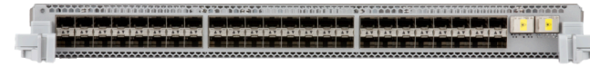
48 port SFP+ for 1/10GbE and 2 port 100GbE SR10 MXP line card - Up to 72 10G ports per line card or 48 1/10GbE ports and flexible 40G/100G - Two MXP ports allow choice of 2 x 100GbE, 6 x 40GbE or 24 x 10GbE
