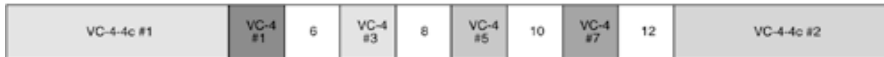
(c) STM-16 (OC-48) signal with two VC-4-4cs (STS-12cs) and four VC-4s (STS-3cs)
