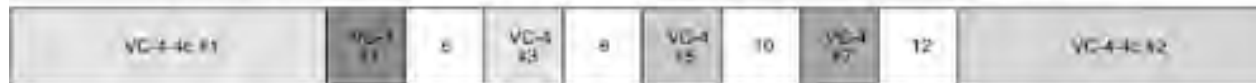
(c) STM-16 (OC-48) signal with two VC-4-4cs (STS-12cs) and four VC-4s (STS-3cs)
