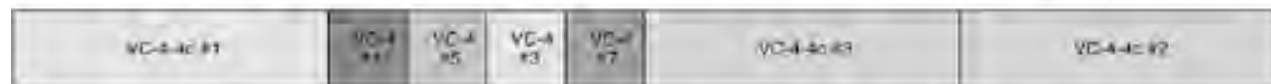
(e) STM-16 (OC-48) signal with three VC-4-4cs (STS-12cs) and four VC-4s (STS-3cs)
