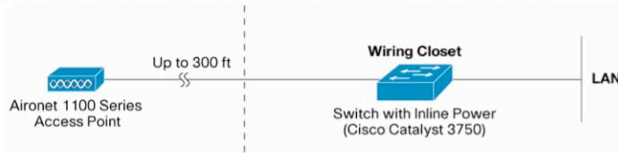
Figure 4. The Cisco Aironet 1100 Series Powered with Cisco Catalyst Switches for Power over Ethernet
