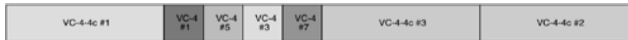
(e) STM-16 (OC-48) signal with three VC-4-4cs (STS-12cs) and four VC-4s (STS-3cs)
