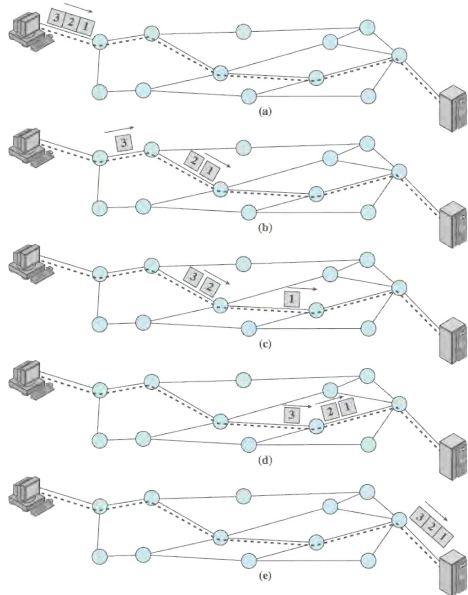
Figure 10.10 Packet Switching: Virtual-Circuit Approach
