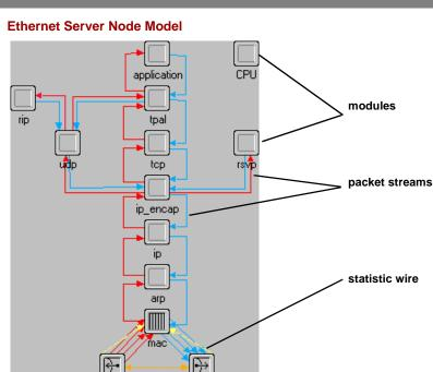
During a simulation, packets sent from a client machine are received by the hub receiver object (hub\_rx\_0\_0) and processed up the protocol stack to the application module. After processing, they are sent down the stack to the transmitter (hub\_tx\_0\_0), then back to the client machine.
